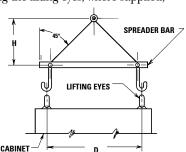
NOTE: When lifting the switch using a spreader bar, height H must be equal to half of distance D.
